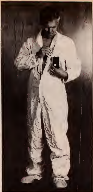
The personal heat stress monitor, developed by Penn State and Westinghouse Electric, clips on to the breast pocket of a worker's uniform.
